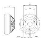
120 W continuous program power capacity 1' horn throat diameter 44 mm (1.7 in) aluminium voice coil Polyimide diaphragm 1000 - 18000 Hz response 108.5 dB sensitivity
